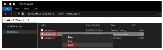
4. Once the installation is complete, connect the camera to the PC using a USB cable, and check that "Photron USB3.0 Real Time Camera" is displayed in the Universal Serial Bus Controller section of the Device Manager.
