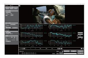
The 6-D Marker is a simple motion capture system that can track and measure 3D image data with six degrees of freedom (X, Y, Z, Roll, Pitch, and Yaw) using only one camera and one 6D-Marker. It's compact structure allows users to measure various automotive tests, including engine vibration and vehicle impacts, which are difficult to analyze with a standard motion capture system.
