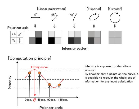
[Schematic view of polarization imaging sensor]
