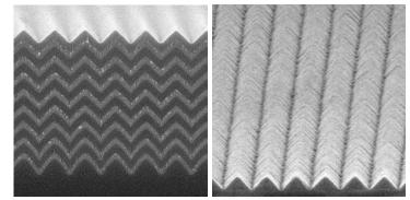
Photonic crystal manufactured with our original auto-cloning technique
