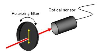
Measure of polarization is made by measuring a change of brightness ]when rotating a polarizing filter.
