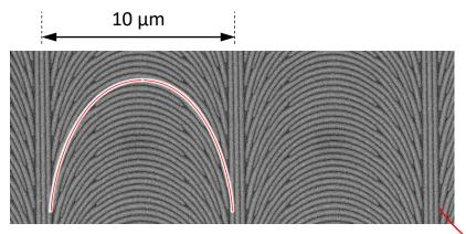
SEM image of the polarization grating surface
