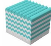
Films material examples:  $SiO_2$ , Si,  $Nb_2O_5$ ,  $Ta_2O_5$ ,  $Al_2O_5$ , etc. = any materials which is available for sputtering deposition process.
