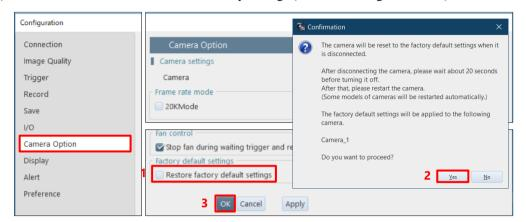
B) Perform PFV4 reset (before connecting the camera).
