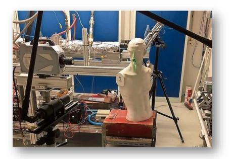
the Photron FASTCAM SA-Z high-speed camera and the distribution of the drops is determined. The advantage of this experimental setup is that it enables completely comparable and reproducible conditions. "A comparison of the droplet distribution for a "coughing" model with and without a mask allows us to assess which masks prevent or at least make it more difficult for certain droplet sizes to spread," says Dr. Schimek.
