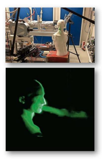
Tests with a model of a head in the laboratory for fluid mechanics. The mouth opening is illuminated by the laser light. A Photron FASTCAM SA-Z high-speed camera records the intensity of the reflected light as the head model "exhales".
