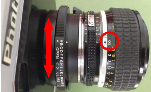
5. Rotate the lens mount barrel until the object comes into crisp focus.
