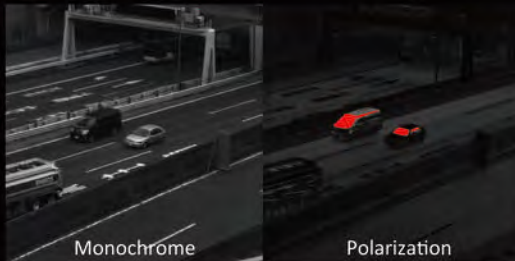
Fig1. Application Example of Window Tracking of Running Vehicles by 1,000fps
