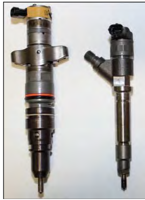
Figure 3. Photograph of the HEUI (left) and CRIN (right) fuel injectors.
